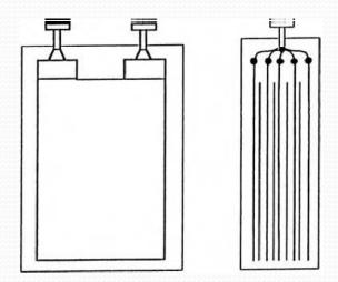
Despite its lowest capacity per unite volume and unit weight, the leadacid battery is the most commonly used battery of the reload types of battery, due to its lowest price in comparison with the other types of batteries.
