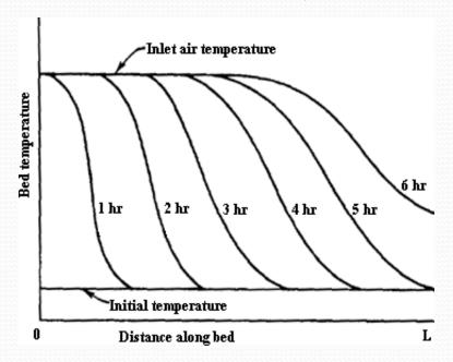
$$\begin{split} (\rho C_p)_f s \frac{\partial T_f}{\partial t} &= -\frac{(mC_p)_f}{A} \frac{\partial T_f}{\partial x} + h_V (T_b - T_f) \\ (\rho C_p)_b (1 - s) \frac{\partial T_b}{\partial t} &= h_V (T_f - T_b) \end{split}$$
