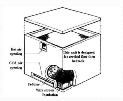
Contemporaneous action of adding and extracting heat could not be effected The high degree of stratification is the major feature of the storage
